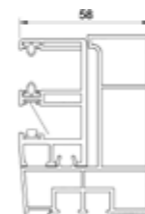
One-sided (PVC) roller guide + MKT* - RS revision from the outside. MK8120 + MK9760
