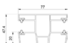
Divisive (PVC) roller guide - RS revision from the inside. MK939
