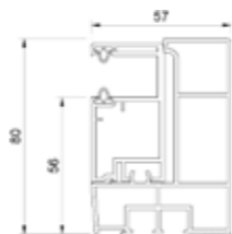
One-sided (PVC) roller guide - RS revision from the outside. MK933 + MK9760
